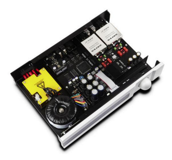
depending on the sampling frequency of 44.1kHz, 48kHz, 88kHz, 96kHz, and so on. For DSD and double DSD files there are two filter choices with different roll off corners and rates. Once the signal is converted to analog it is buffered by proprietary dual-differential class A output stages (for the balanced outputs only) contained in packaged modules. The implementation of all this very high performance circuitry in the chassis is first rate.
